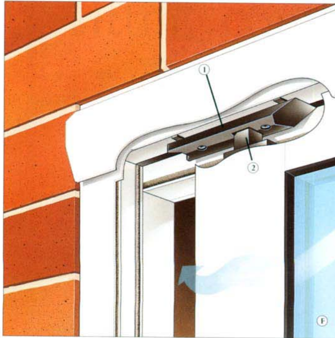
Ⓕ All sliding patio door frame heads are fitted with (1) anti-lift blocks to prevent the door panels being lifted out of the frame, and (2) optional shoot bolts which allow the door to be held partially open for the flow of fresh air but stops toddlers or pets getting out. Our 'anti-slam' feature avoids damage to the locking mechanism should the door be slammed closed.
